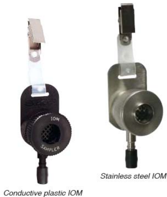
Figure 2 IOM conductive plastic (left) and stainless steel (right) sampler (source: http://www.skcinc.com/instructions/37372.pdf )
