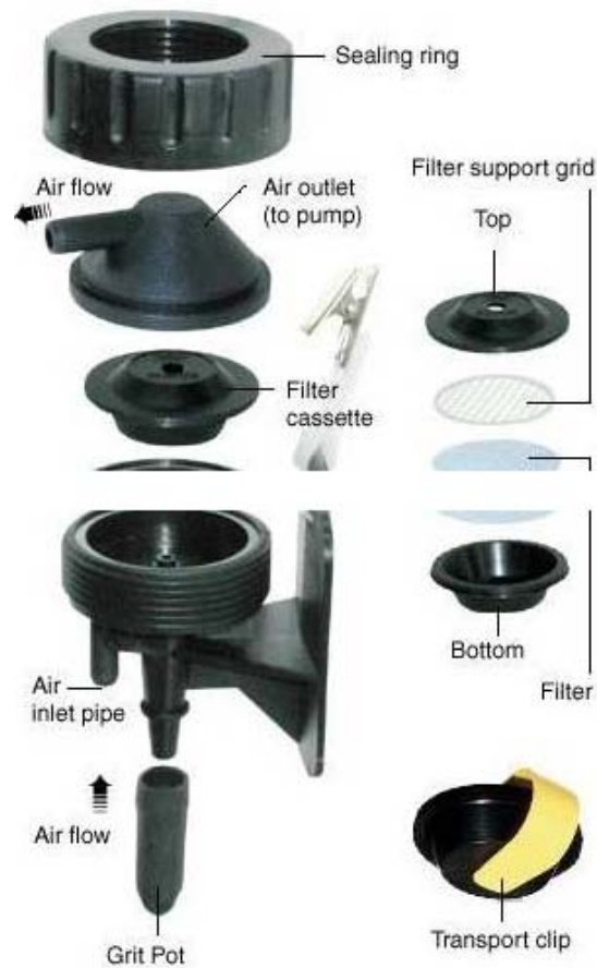
Figure 3 Casella Measurement plastic cyclone components (right)
